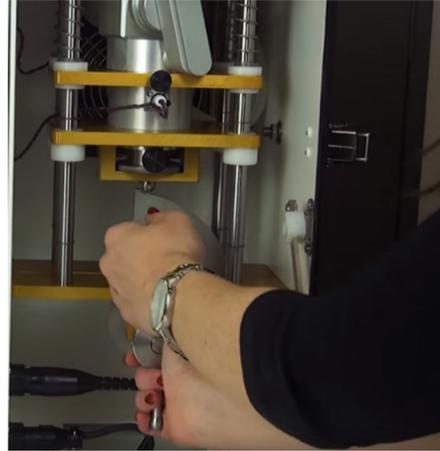
**Step 7.** The filter holder assembly and filter cassette is installed prior to shipment. Inspect the filter housing and filter cassette for obvious missing pieces or damage. Confirm the presence of O-rings inside the upper and lower filter housings where they contact the filter cassette. Ensure the housing interior is clean and free of debris.
