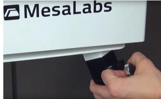
**Step 2.** Attach the AC power supply to the rear of the unit underneath the fan cowling. Use the plate on the AC power supply to hook it to the rear of the instrument. Run the female, three-pin connector underneath the sampler to the hole in the sampler case near the front on the right side. Open the main door on the PQ200 and feed the connector through the hole and attach it securely to the upper of the two connectors.
