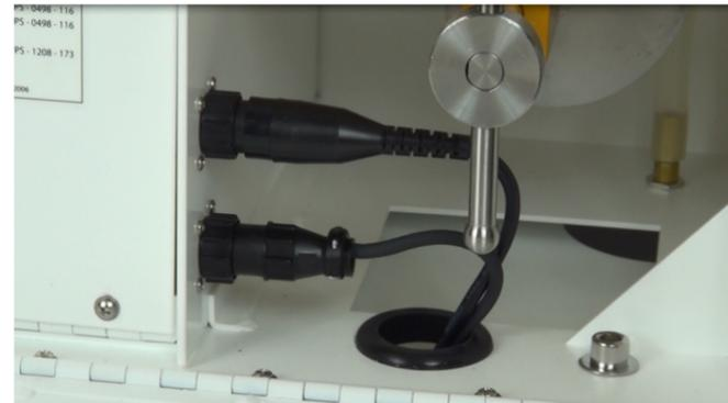
**Step 3.** Attach the external temperature gauge to the rear of the unit. The attachment points are on the fan cowling itself. Position the temperature gauge assembly so that it sits above the top of the sampler case. Screw the connectors firmly into the attachment points. Run the cord with the three-pin connector underneath the sampler case and through the hole, just as with the power connector, and attach it to the lower of the two connectors.
