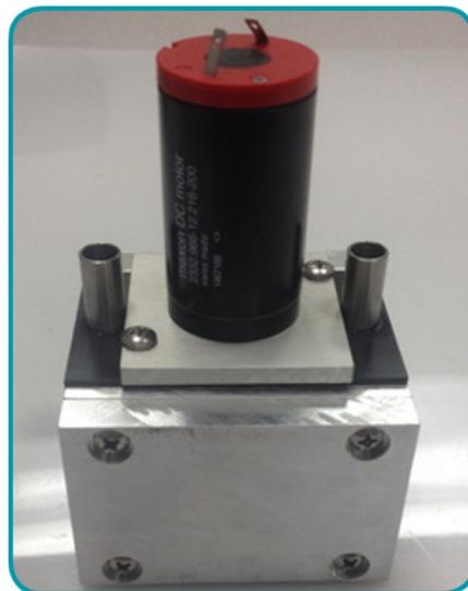
**Step 1:** To start rebuilding your pump, remove the two screws that secure the motor to the pump body. The motor assembly can now be pulled away from the pump body. Inspect the eccentric bearing for looseness on the shaft. Inspect the bearing for smooth rotation and absence of play. If these components are in good condition, then wipe the bearing clean with a fresh, lint free cloth and re-lubricate with light grease. Set aside for reassembling.
