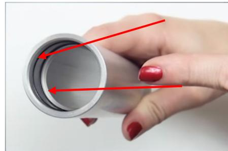
**Step 5.** Confirm the presence of two O-rings on the bottom side of the size selective inlet that mates with the downtube. Install on top of downtube. The water collection hardware is packed separately to avoid shipping damage. Locate and attach to the side of the size selective inlet.
