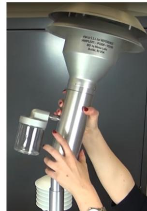
**Step 6.** The VSCC assembly is installed prior to shipment with model PQVSCC. Open the VSCC and filter assembly inside the PQ200 sampler case by carefully rotating the handle counterclockwise using both hands. Inspect the VSCC for obvious missing pieces or damage. Ensure the interior of the VSCC is clean and clear of any debris.
