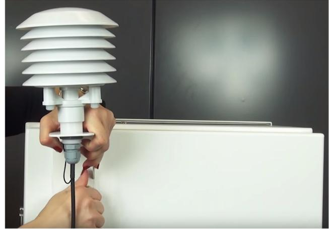
**Step 4.** Confirm the presence of two O-rings on the bottom end of the downtube that mates with the open tube on the top of the sampler case. Ensure the interior of the tube is clean and clear of any debris. Install downtube on sampler.
