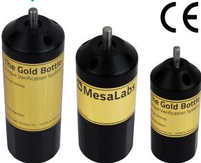
The Gold Bottle is constructed with high energy permanent magnets and can be pre-set at the factory to a customer specified torque value. Each Gold Bottle is labeled with its exact torque rating, serial number and repeats to an accuracy of  $\pm$ 0.2 inch pounds.
