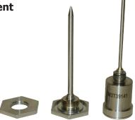
Keeps the body of the data logger out of the container during the process.
