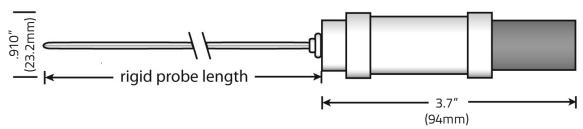
Probes available in the following lengths: **Rigid:** 2'' (51 mm), 3'' (76 mm), 4'' (102 mm), 5'' (127 mm), 6'' (152 mm) Rigid probe diameter: 0.125''/3.2mm or .188'' (4.76mm) available
